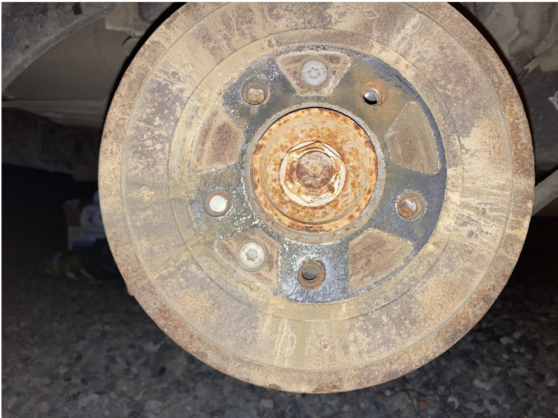
Figure (4.25) 3 bolts sheared off where the wheel attaches to the car.
